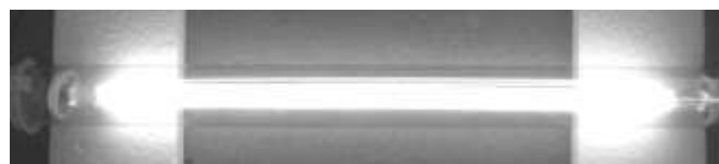
(B) 10 coil-EEFL lamps in a vacuum-sealed sheath tube
