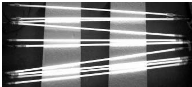
(A) 10 parallel connection of coil-EEFL lamps under DC 3kV
